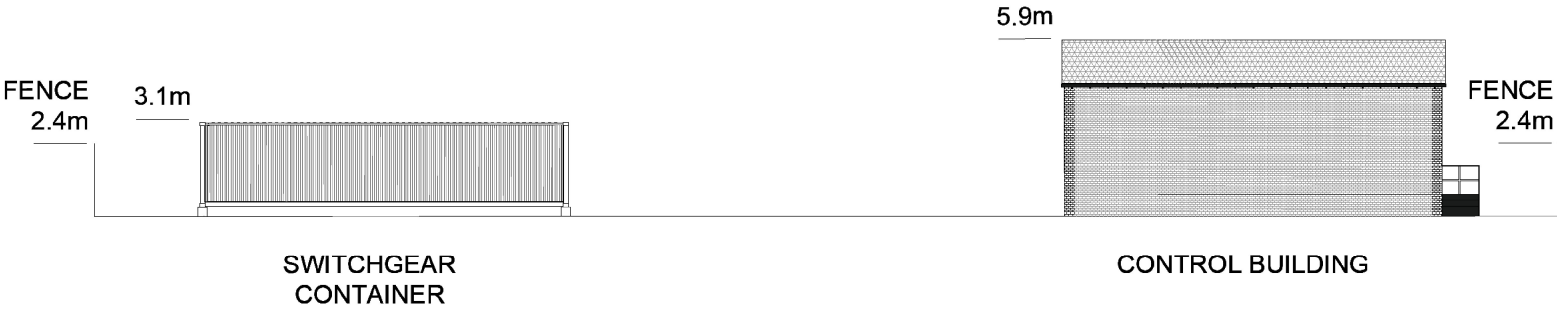
S2 - SWITCHGEAR COMPOUND ELEVATION 2
