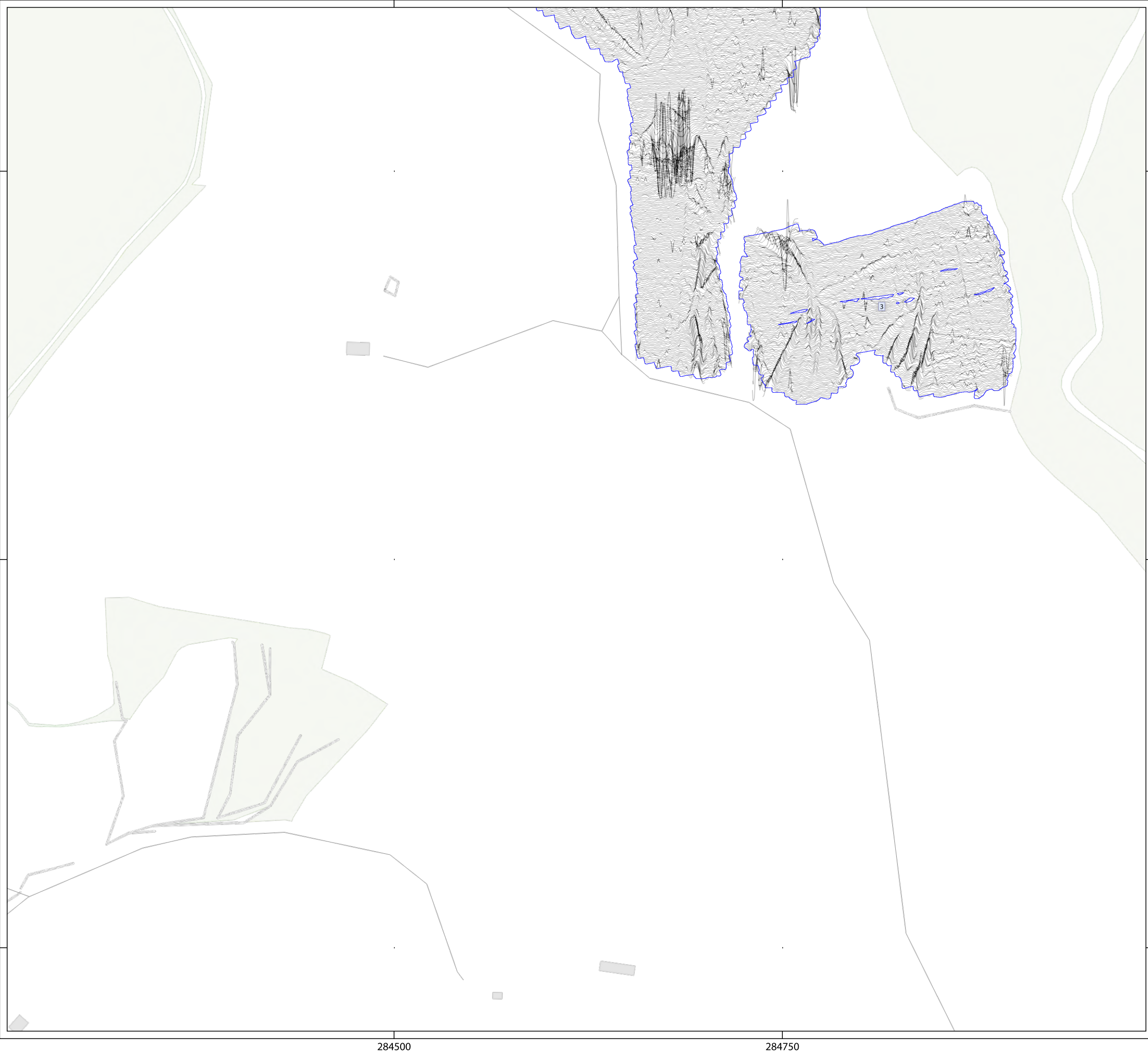
Illus - 21 XY trace plot of minimally processed magnetometer data; Sector 2
